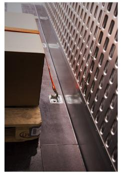
**INTEGRATED LASHING RINGS** Talson trailers are equipped with 26 lashing rings, 13 on each side, discreetly integrated into the vehicle floor to anchor heavy weights for maximum load security.
