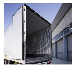
**FLOOR PROTECTION PLATE** The entrance of the trailer is lined with a 600 mm, non slip steel plate.
