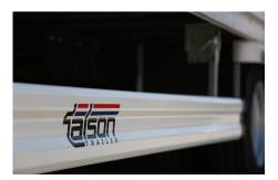
**SIDE UNDERRUN PROTECTION** The side underrun rail is a lateral protection device made of KTL coated steel profile which can be folded upwards for easier access to vehicle when needed..
