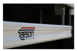
**SIDE UNDERRUN PROTECTION** The side underrun rail is a lateral protection device made of KTL coated steel profile which can be folded upwards for easier access to vehicle when needed..
