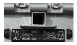
**SPECIAL FORKLIFT SPACE** Thanks to the special forklift space, the forklift can be connected to the trailer and transported to the location of the loading and transportation operation.
